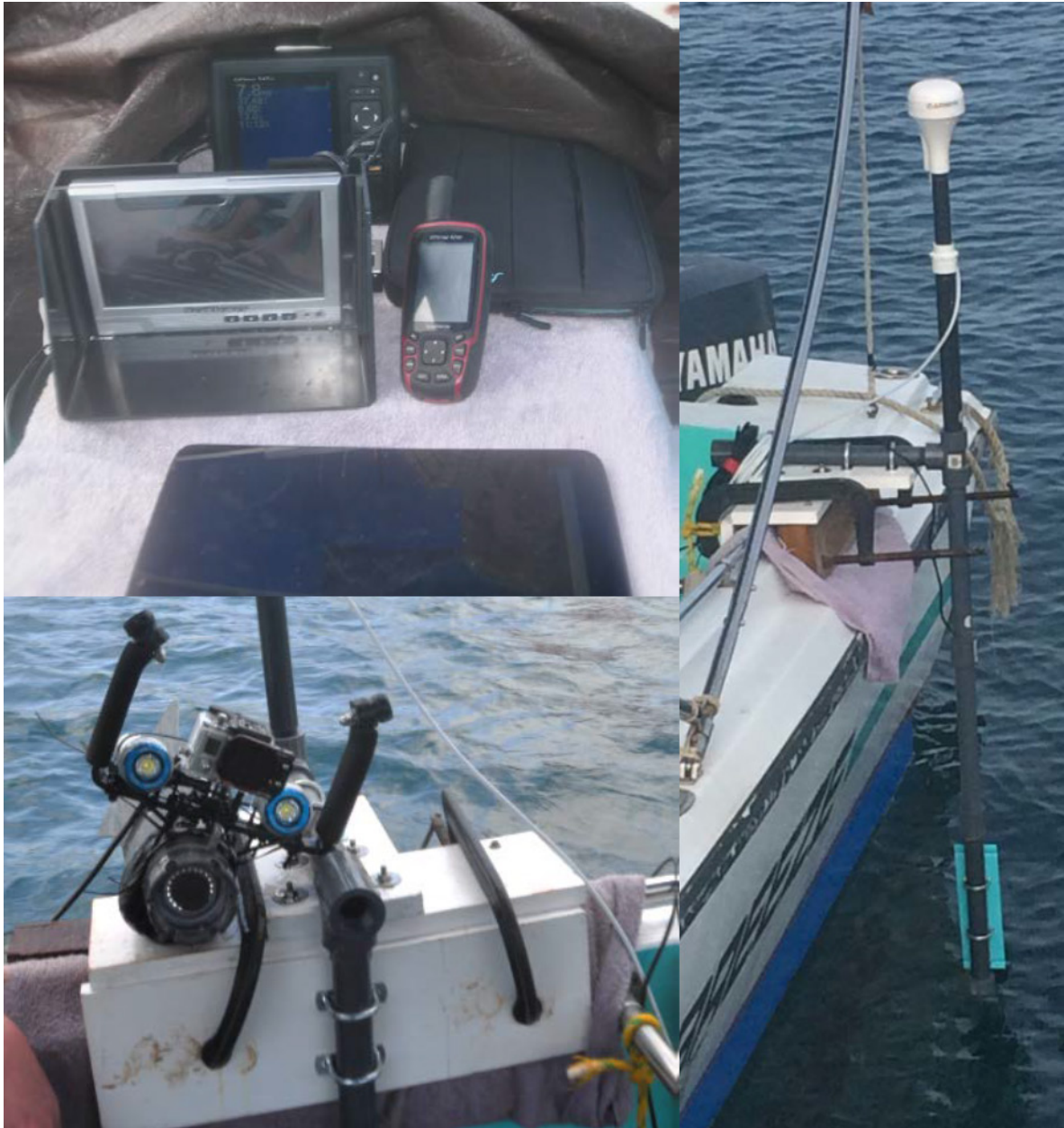
Figure 5. Instruments used for collecting field samples in 2016 and 2019 included a GoPro Hero 4 camera with a red filter affixed to a GPS-referenced SeaViewer Sea-Drop 6000 HD (Tampa, FL, USA) underwater video camera with a 30 m vertical cable and a Garmin GPSMAP 547xs transducer. The Seaviewer provided a live video feed used for obstacle avoidance while the GoPro captured high definition video footage of benthic habitat along each transect. GPS points were registered at beginning and end of each transect to allow for georeferencing of habitat information. The transducer assembly collected depth at 3 points per second with GPS antennae. High resolution imagery converted to MBTile format and loaded into the Locus Pro application
